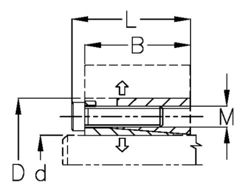
$\begin{array}{lll} \text{B mm} & = 28.0 \\ \text{d H8 mm} & = 22 \\ \text{D mm} & = 47 \\ \text{Fit tolerance} & = \text{Aksel h8, Nav H8} \\ \text{F kN torque} & = 41 \\ \text{L mm} & = 34 \\ \text{M mm} & = \text{M6} \\ \text{P N/mm2 surface pressure on shaft/hub} = 140 \\ \end{array}$
